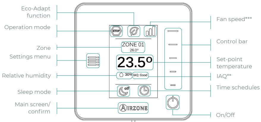
Only in the case of a wireless Think thermostat | Communication frequency: 868 MHz
